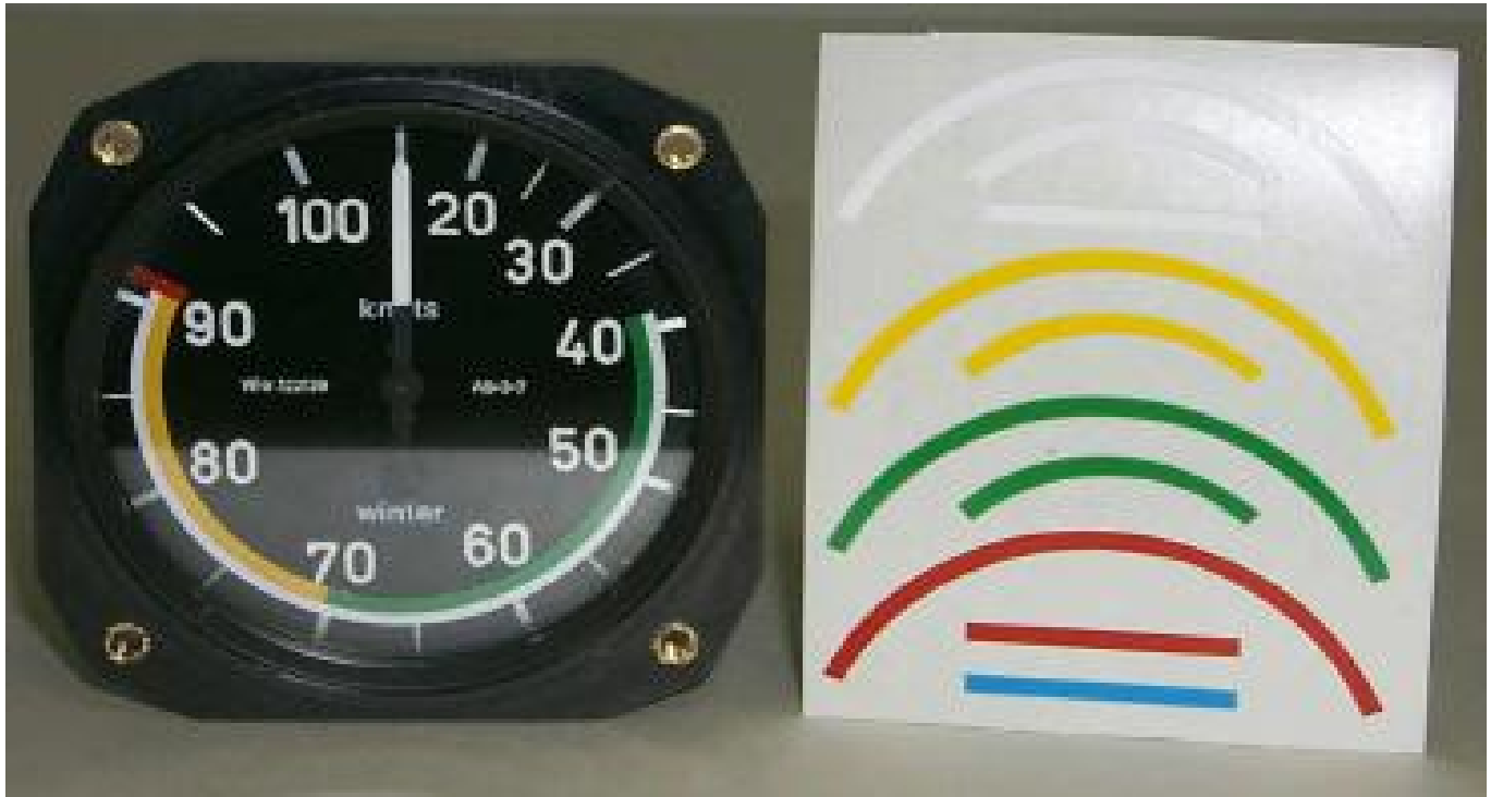
Fig.5.6.1C: The color marking kit will be used to satisfy the FDR regulations for airspeed indicator by highlighting the different tolerable ranges in airspeed for the aircraft.
