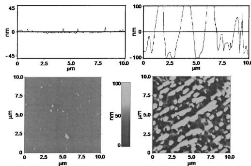
FIG. 2. AFM images of the crater bottom after completion of the depth profile analysis. The left panel (a) shows the image acquired after 15 keV  $C_{60}^+$  bombardment and the right panel (b) shows the image acquired after 15 keV  $Ga^+$  bombardment. The rms roughness was calculated using the line scan data shown above the respective images. The rms roughness of the surface before bombardment was about 8 nm.
