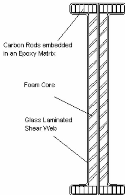
Figure 2: Completed Spar
