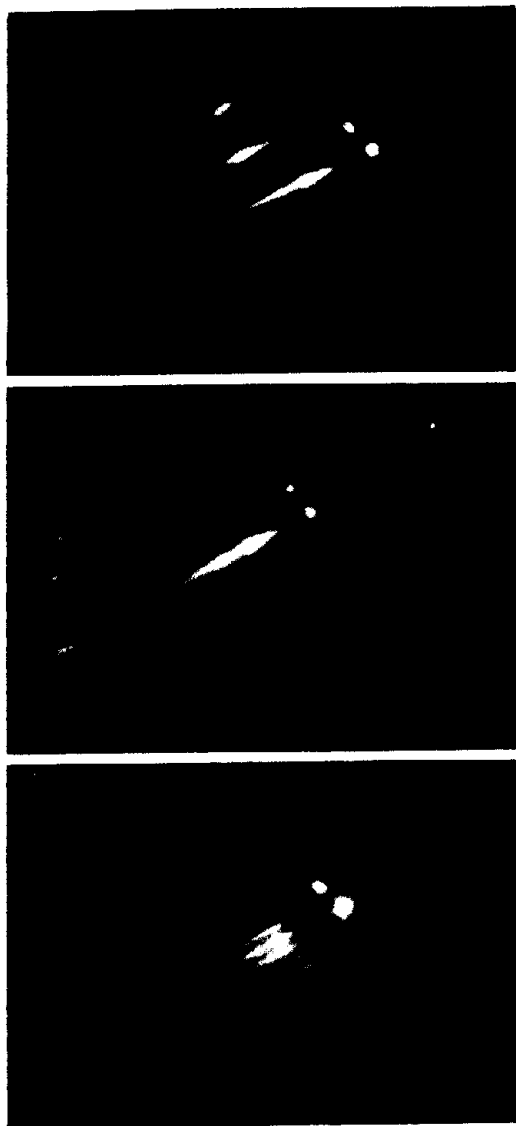
FIG. 1. Room-temperature RHEED pattern of (2 \times 4) GaAs (100) in the [110] direction (top), the [100] direction (middle), and [\bar{1}10] direction (bottom).
