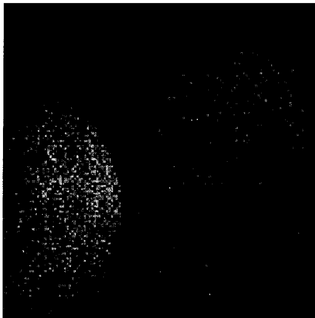
Figure 7. Postionization image of PBA + desorbed from Ag beads using 60 ns (2 nA) ion gun pulses with 40 shots per pixel ( 2.2 \times 10^{12} Ga + ions/cm 2 ). The PBA molecules are ionized with 267 nm, 250 fs laser pulses at a laser power of 1.4 \times 10^{11} W/cm 2 . The 128 pixel \times 128 pixel image was collected from a 150 \mu m \times 150 \mu m area.
