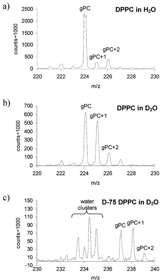
Figure 6. (a) Spectrum of freeze-fractured DPPC frozen in  $\text{H}_2\text{O}$ , (b) spectrum of freeze-fractured DPPC frozen in  $\text{D}_2\text{O}$ , and (c) spectrum of freeze-fractured D-75 DPPC in  $\text{H}_2\text{O}$ .  $1 \times 10^{11} \text{ In}^+$  ions/ $\text{cm}^2$  with 15-kV beam voltage was used in each experiment.
