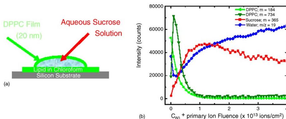
Fig. 2. (a) Schematic representation of DPPC–sucrose frozen multilayer structure, illustration not drawn to scale.; (b) Depth profile plot of DPPC molecular fragment  $C_5H_{15}NPO_4^+$  ( $m/z = 184$ ), DPPC molecule  $C_{40}H_{81}NPO_8^+$  ( $m/z = 734$ ), sucrose–sodium adduct  $C_{12}H_{22}O_{11}Na^+$  ( $m/z = 365$ ), and hydronium water  $H_3O^+$  ( $m/z = 19$ ) vs.  $C_{60}^+$  ion fluence.
