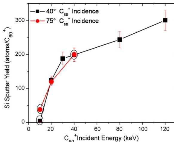
**Fig. 1.** Silicon sputter yield as a function of  $C_{60}^+$  incident energy. The black squares represent the yield at  $40^\circ$  incidence and the red circles represent the yield at  $75^\circ$  incidence. The experimental error is  $\pm 10\%$ . The yields were calculated using AFM to determine the volume removed from a Si crystal bombarded to a fluence of  $\sim 2.0 \times 10^{16}$   $C_{60}^+$  per  $\text{cm}^2$ . The data for the points circled are shown in detail in Fig. 2a–c.
