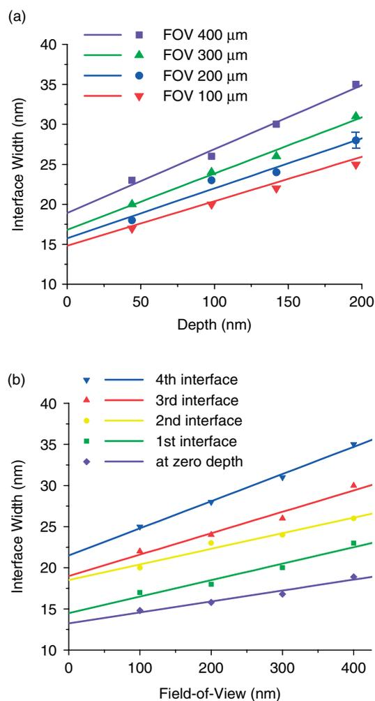
**Figure 3.** Interface width extracted from depth profiles accumulated over different gating area vs (a) interface depth and (b) size of the gating area.
