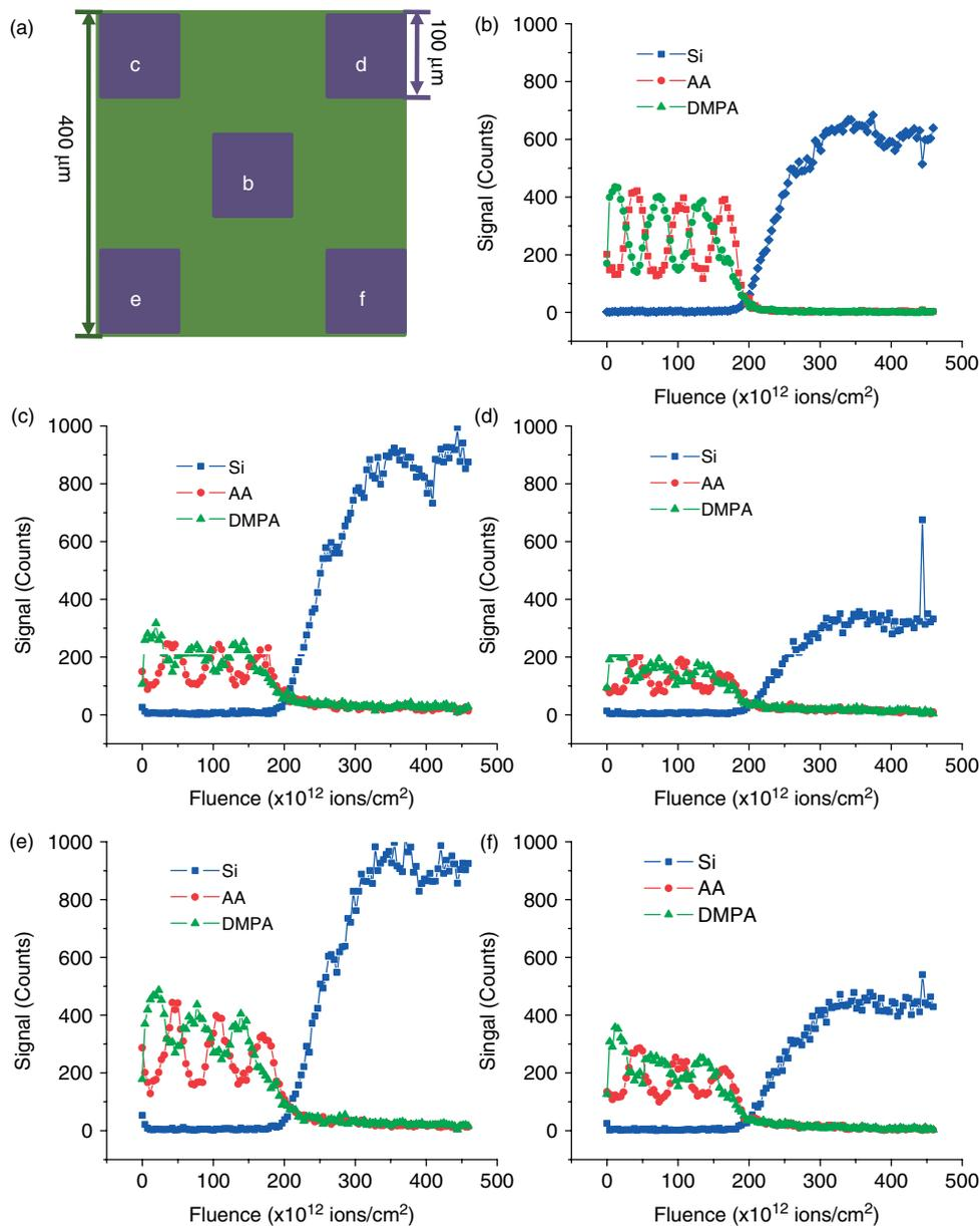
**Figure 1.** (a) Schematic drawing (ion beam impinging from the bottom) to show the location of gating area used to extract depth profiles displayed in (b)–(f) within the original three-dimensional dataset.
