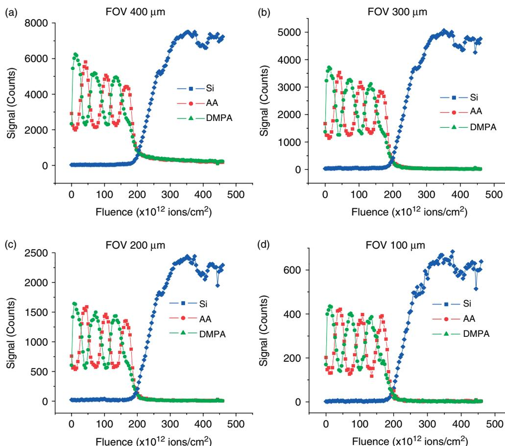
**Figure 2.** Depth profiles extracted from the 3D image stack using different gating area (FOV) centered within the sputter eroded crater.
